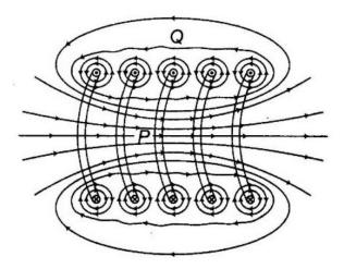
13. (i) Behavior of magnetic field lines when diamagnetic substance is placed in an external field.
